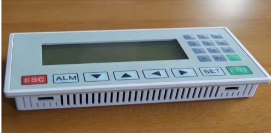
Figura 6. Pantalla HMI. (2018) Recuperado de: https://m.es.dhgate.com/product/1-pcs-text-display-op320-a-hmi-panel-display/446719654.html
