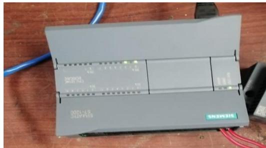
**Imagen No. 4** CPU 1211C AC/DC/RLY SIEMENS
