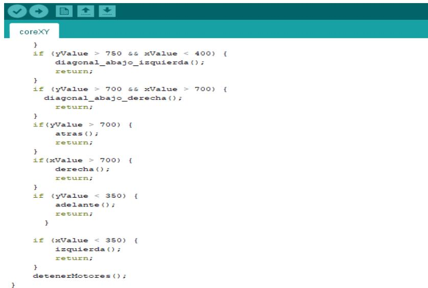
The image shows a code editor window with a teal header bar containing icons for save, undo, redo, and search. The code is written in C++ and is titled 'coreXY'. It defines a function that checks the joystick's x and y values to determine movement directions: diagonal down-left, diagonal down-right, back, right, forward, and left. If none of these conditions are met, it calls 'detenerMotores()' to stop the motors.
