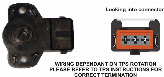
Figure 3 – Throttle Position Sensor
