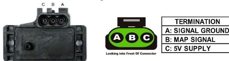
**Figure 5 – Manifold Absolute Pressure Sensor and harness Termination**
